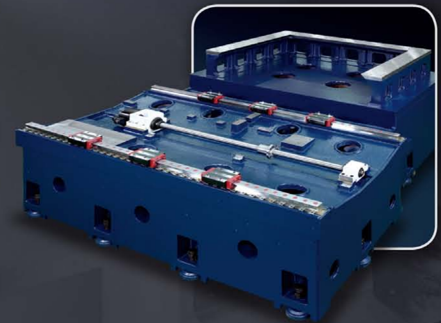
Machine design by computer FEM analysis to achieve high rigidity base, provide high position depth cold C1 class ball screw, with roller type linear guide way use three support block to provide accuracy machine positioning & cutting.
